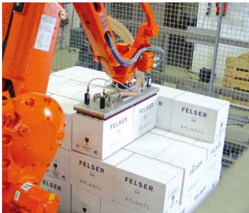
Palletizing robot with vacuum suction grippers
