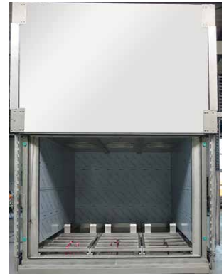
Automatic lift gate
