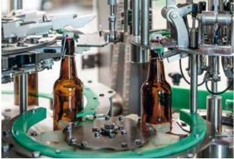
The continuous closing operation with mechanically guided, smooth motion sequences allows for low-wear, optimum closure performances.
